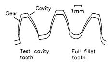
Fig. 5 Teeth of the cavity and molded gear
