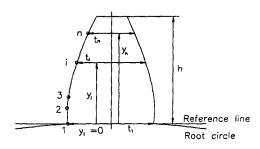
Fig. 1 Measurement of tooth heights and thicknesses
