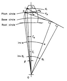
Fig. 2 Tooth geometry
