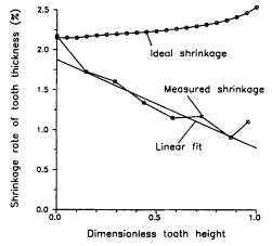
Fig. 3 Variation of shrinkage rate with dimensionless tooth height in the test cavity
